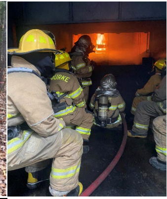
Students observe a fire in the Flashover simulator to learn about fire behavior.
